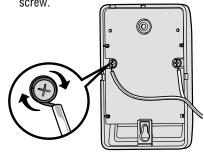
**PRE-WIRED INSTALLATIONS:** Choose any two wires to connect, but make note of which wires are used.
