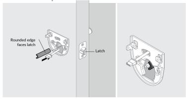
STEP 6 - Disassemble interior assembly and load battery pack
