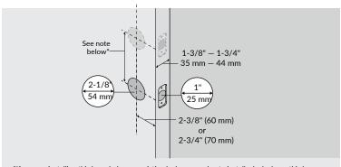
$^*$ If you are installing this lever below an existing lock or you plan to install a lock above this lever, make sure that the distance between holes is at least 6-1/2 " (165 mm).
