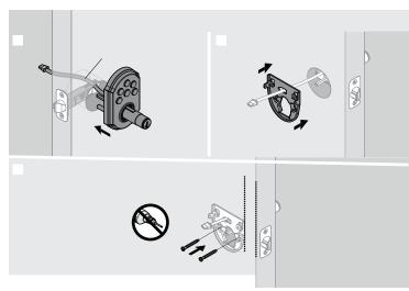
**STEP 5 - Install spindle**
